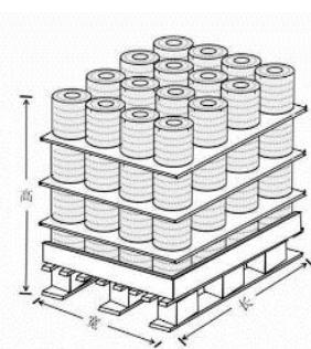
Please store the glass fiber products in a dry and cool environment, with recommended temperature control between 10-30°C and humidity control between 50-75%. Stack pallets no more than 2 layers high.
